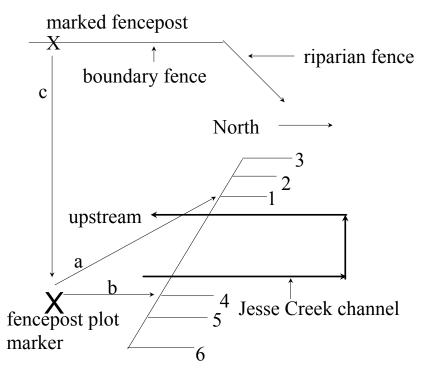
a - transect #1 footmark stake located 28.3 m (across channel loop) at 310 degree bearing from fencepost
